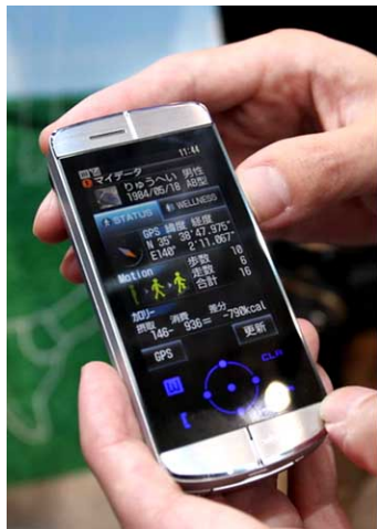
Fig. (11). Wellness phone prototype, measuring one's body fat, heart rate, bad breath and footsteps [48].
