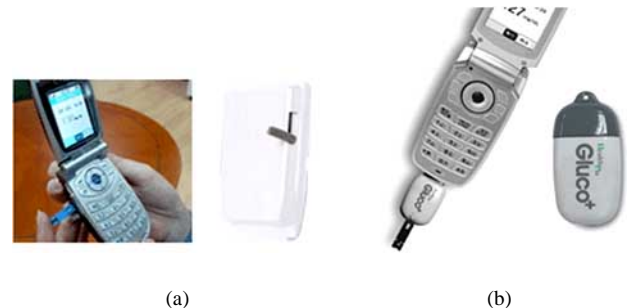
Fig. (5). (a) Diabetes Phone, Convergence products of mobile phone and glucose meter; (b) Regardless of phone model, it works with mobile phone through the phone connector [35].
