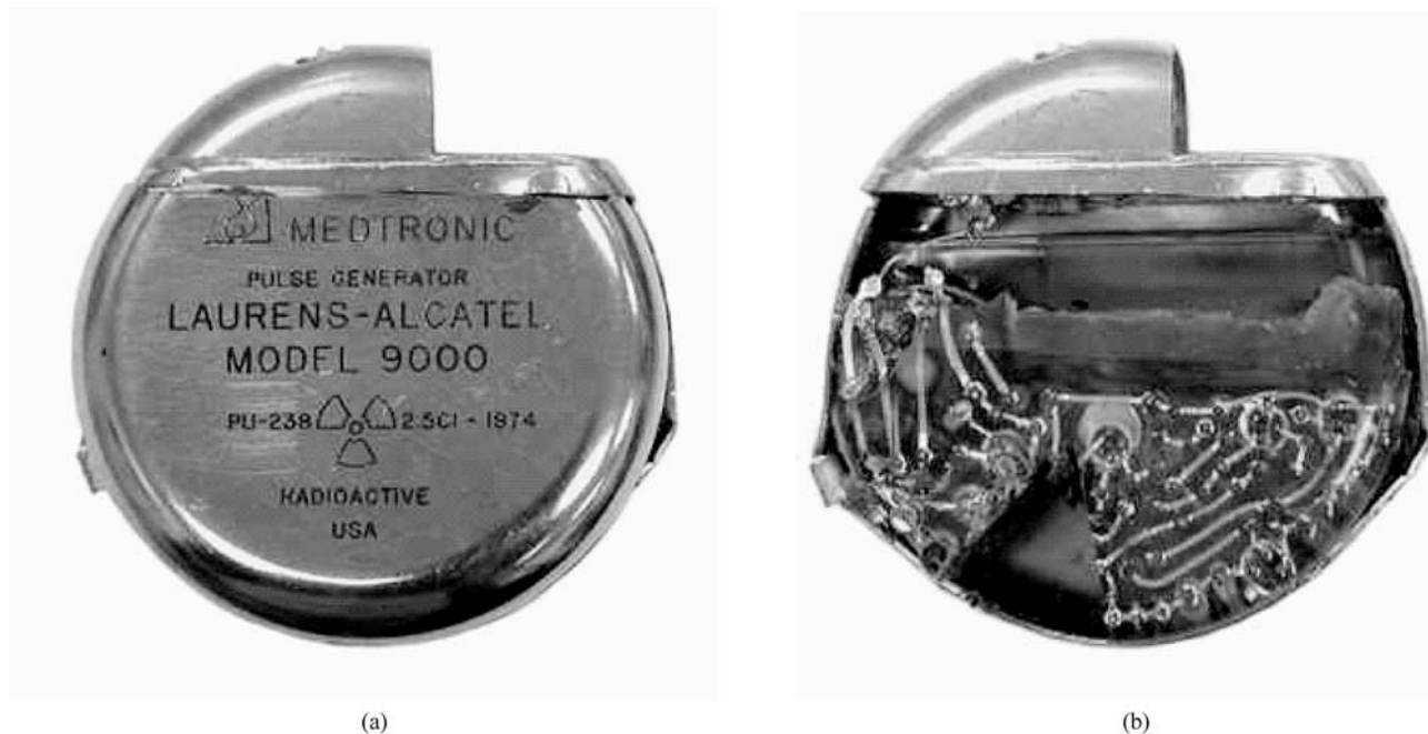
Fig. 6 Nuclear pacemaker developed for Medtronic used a tiny slug of Plutonium 238 [33] (a) A nuclear pacemaker; (b) the same one with plutonium removed
