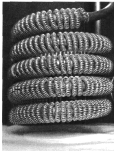
Fig 3 Evaporator made by copper tube coiled with small spring
