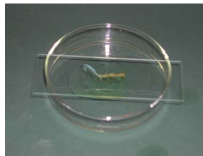
Fig. 12 An optical image for two connected wires with different components. The junction represents a thermal couple.
