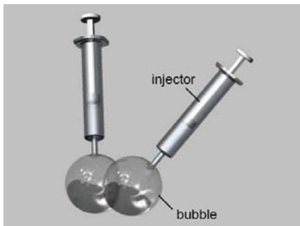
Fig. 2 Sketch for using two injectors to blow bubbles and drive them to contact to each other for the micro fabrication.
