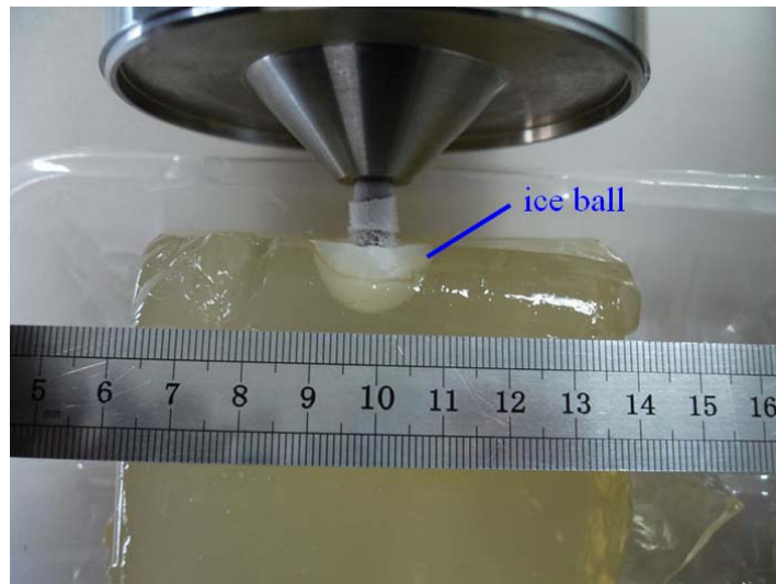
Figure 4. Ice ball generated by the TE system in tissue phantom ( I_s = 3A , Q_f = 2.5g/s , T_i = 20^\circ C )
